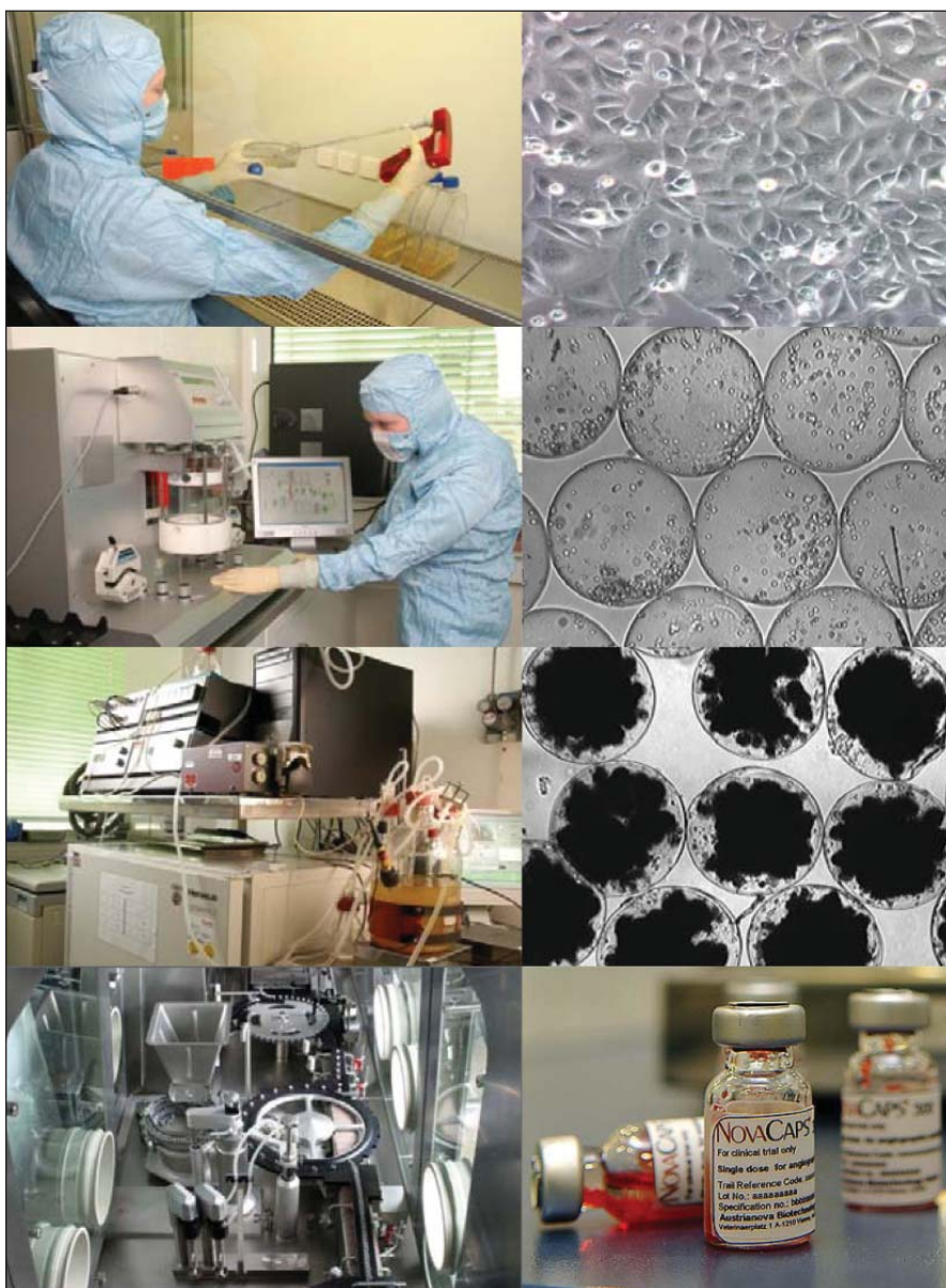
Figure 5. Various steps in the continuous process required to produce NovaCaps®. After unfreezing a vial from the working cell bank, cells are cultivated (top two panels), harvested, and encapsulated 23 using a custom-built GMP-compliant encapsulation device (left, second panel). The encapsulated cells (right, second panel) are washed and transferred to a biofermenter in cell culture medium (left, third panel). They grow within the capsules to fill the available space, but without breaching the confines of the capsules, thereby attaining a confluent state in three dimensions (right, third panel). They are then aliquotted (left, bottom panel) into vials (right, bottom panel) and frozen at -80^{\circ}\text{C} .
